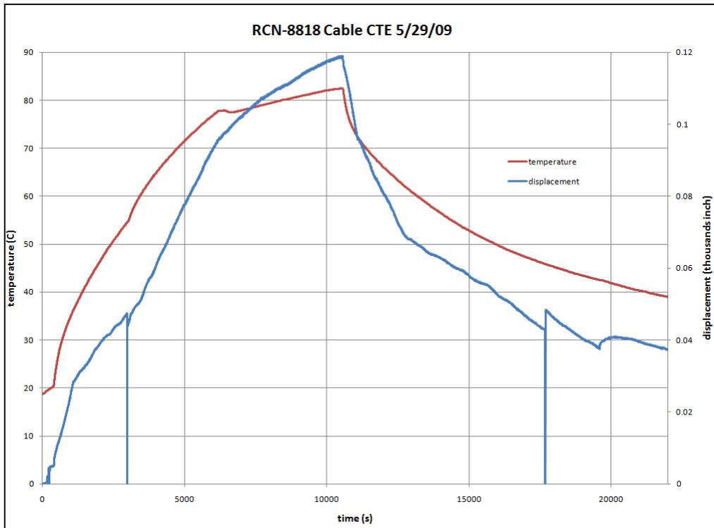
**Figure 2. CTE testing flight RCN-8818 Gore composite cable**
